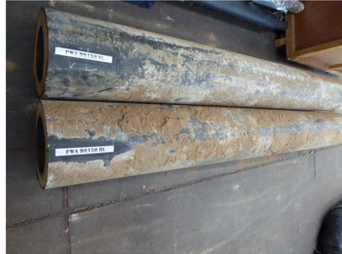
Straight pipes FWA before material testing according to EN 253, Source: AGFW
