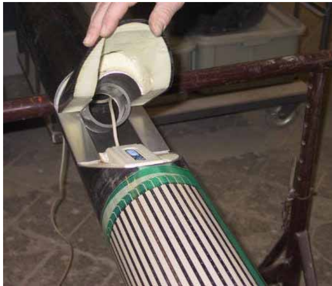
FIG. 4 — Pressure sensor, data logger and cable mounted on the pipe
