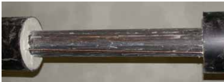
Figure 2. Space for simulated moisture faults.
