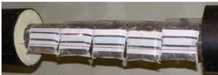
Figure 3. Water filled bags. Each bag contains approximately 90 ml water, is approximately 80 mm wide and fills up the 18 mm space between the wire and the pipe.
