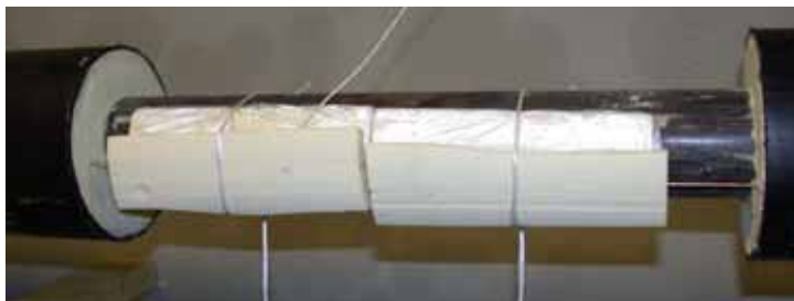
Figure 4. Partially water filled PUR foam. The foam pieces are shaped as “quarter shells”, covering one fourth of the service pipe’s circumference, with a thickness in the radial direction of 18 mm. The picture shows two wet 190 mm long foam pieces wrapped in plastic foil arranged to a total length of 380 mm. The wet PUR pieces had a moisture content of 50 - 58 % (percentage by volume). Two dry foam pieces are placed externally. The plastic foil is used to prohibit electric conduction between the wire and the service pipe.
