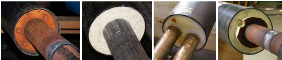
Figure 3. Examples of pre-treatments of pipe ends: A) Normally stored. B) Clean cut. C) Polyethylene end seal. D) Staircase surface profile.
