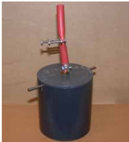
Figure 5. Test rig for water permeability measurements. H is the cylinder's total height, T is the thickness of the lid inside the cylinder, L is pressurised air volume, V is the water depth when the test starts, P is the PUR samples thickness and B is the height of the volume open to the ambient air.
