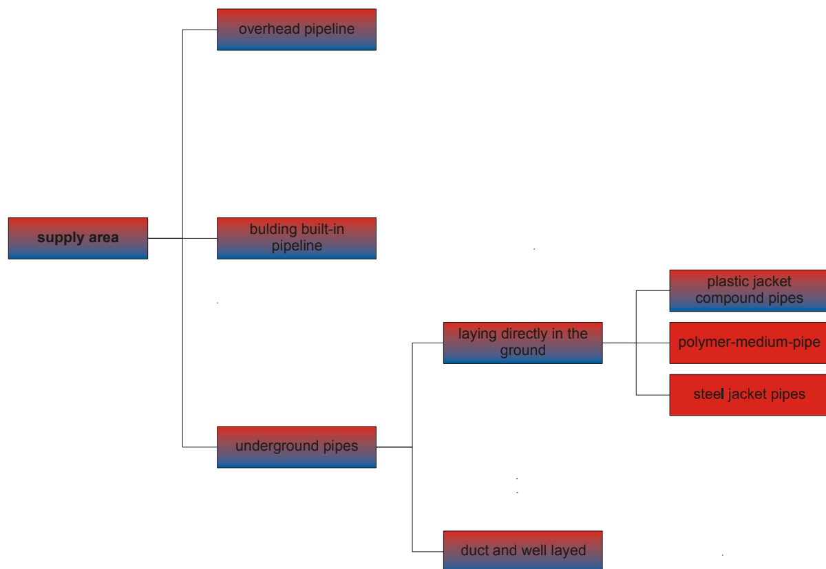
Picture 1: Over view about the laying methods (blue: application of Polyurethane with cooling pipes; red: application of Polyurethane with heating pipes)
