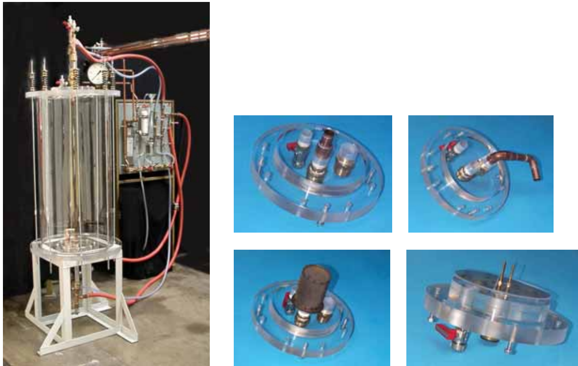
Figure 1: Test rig "Plexiglas storage tank model" – tank design (left) and inflow devices in the removable lids (right)
