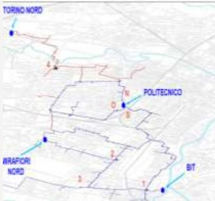
***IREN and AES have jointly realized a project of development of the district heating network supplying 410.000 inhabitants (45%) of Torino based on gas fired CHP.***
